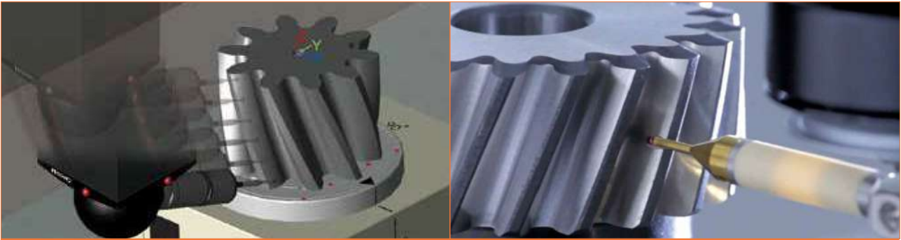
4 Axis technology supporting high-speed scanning
