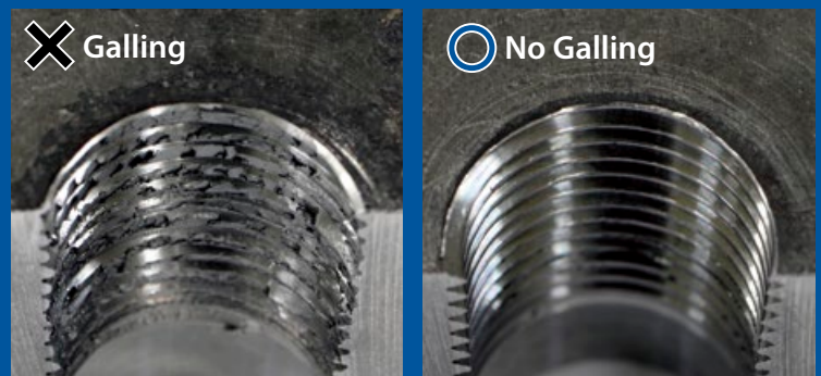
SS400材での加工イメージ Image to process taper pipe thread in SS400 material
